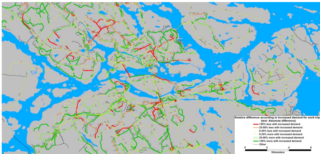
Figure 29: Relative flow difference between 7 and 8h with regards to increased work trips demand.
